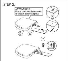
Ensure the word 'Outward' on the backrest post (6) is facing outward and the text is the right way up. Please note the backrest post may initially be tight to assemble.
